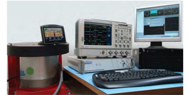
Typical test system using a GSS6700 with SimAUTO driving a rate table & producing wheel ticks
