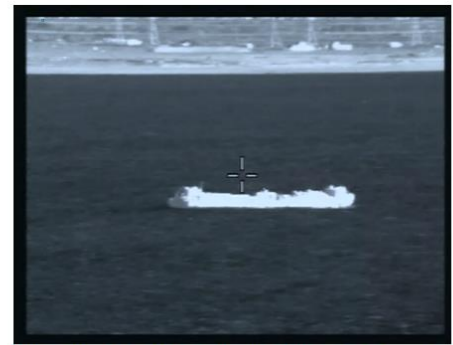
Recognising vessels using Thermal imager Camera (Targets ~10km)
