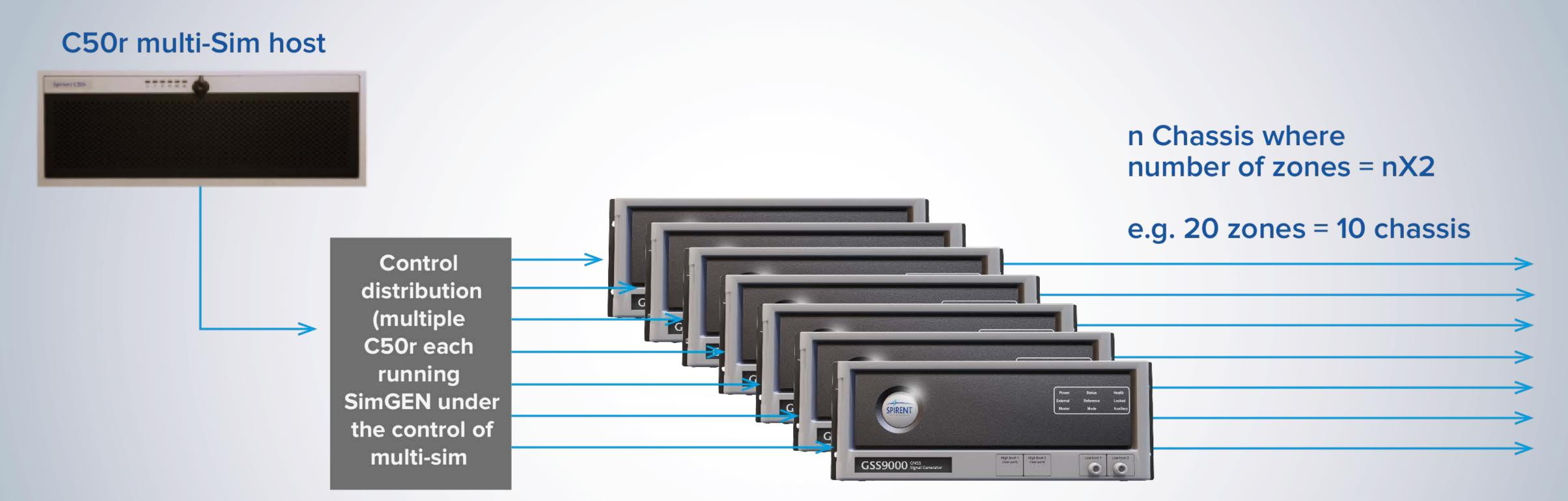
Each dual RF chassis drives two zones with multiple banks behind each RF output
