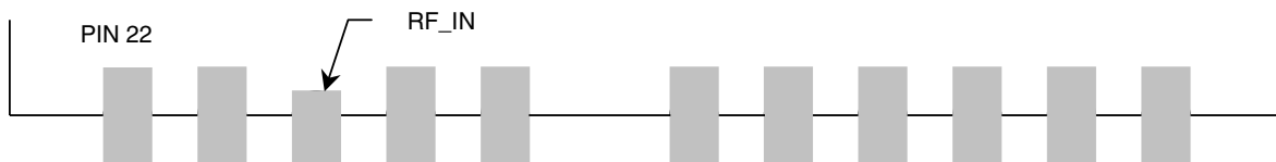
Figure 4 Solder Pad Size and Placement
